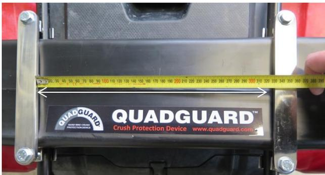
Tighten the hooks with a torque wrench to 8 newton meters, which is adequate for a secure mount. Over tightening may bend the hooks or the carrier, and also damage the "QUADGUARD"
